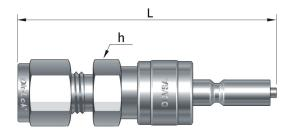
**DV**: Stem has a valve **SV**: Stem has no valve
